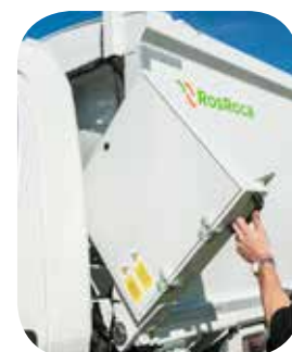
6 Electrical control panel in an easily accessible place.
