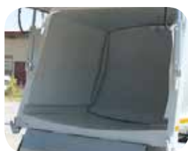
2 Sloped floor with side ejector guides.
