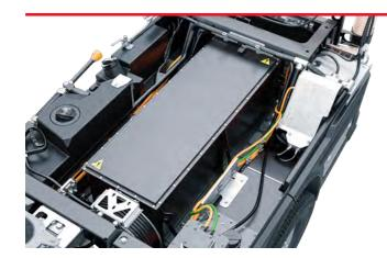
Specially designed Bucher Battery Pack with superior lifetime and no memory effect. Made with high quality automotive prismatic Li-ion NMC cells, managed through an automotive battery management system, the battery is placed in a shock, water and dust-proof case. The Bucher Battery Pack is maintenance-free and has a sophisticated repair concept for maximum safety. Due to the electric drive concept of the sweeper, maintenance and service costs in general are kept very low.
