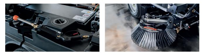
High pressure water system with hand lance 120 bar high pressure system for cleaning walls, staircases, posts, handrails and such, as well as the sweeper. The hand lance, water hose and an automatic reel are easily accessable via the flaps on the hopper.
